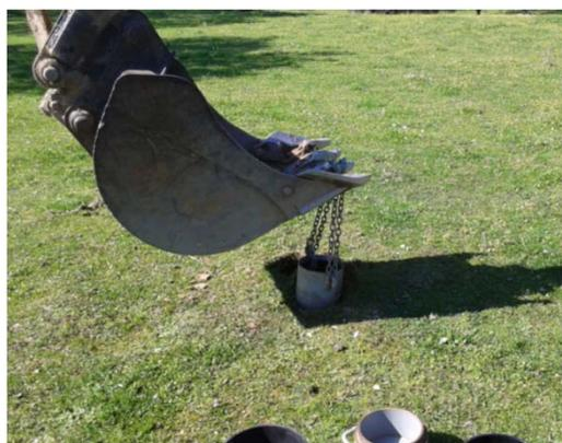
Collection of intact soil cores for the Climate Chamber Experiment (Portugal)
